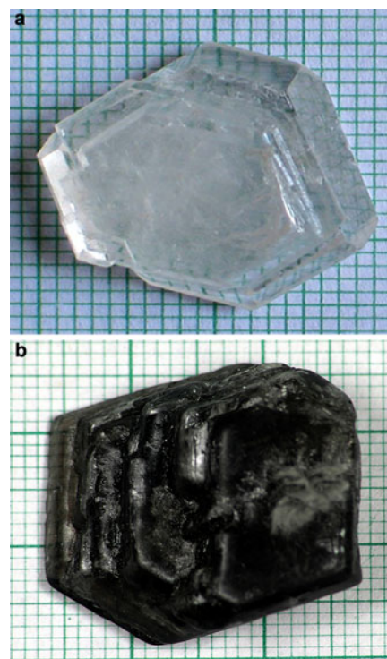
Fig. 1 Photographs of KHP as-grown crystals a pure and b 1 mol% \text{OsO}_4 doped
